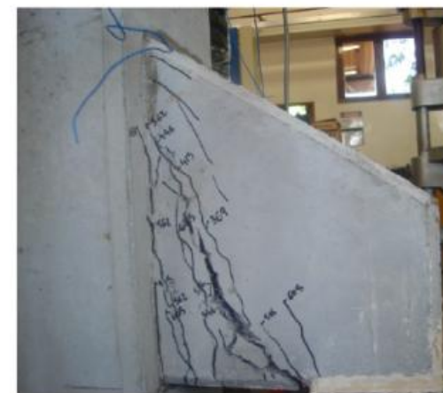
b) Monolithic corbel without secondary reinforcement and with SFRC (Mono1-A-1 (sample1))
