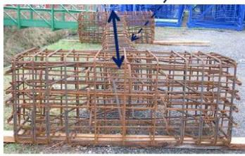
Forces in the struts and strains in the steel reinforcements allows to deduce accurately stresses in concrete just before the first cracking.
