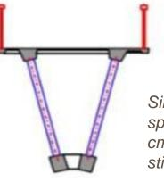
Single 60 meter long span with an only 3 cm thick deck with stiffening ribs.
