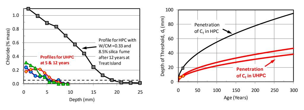
Chloride profiles: UHPC versus HPC
