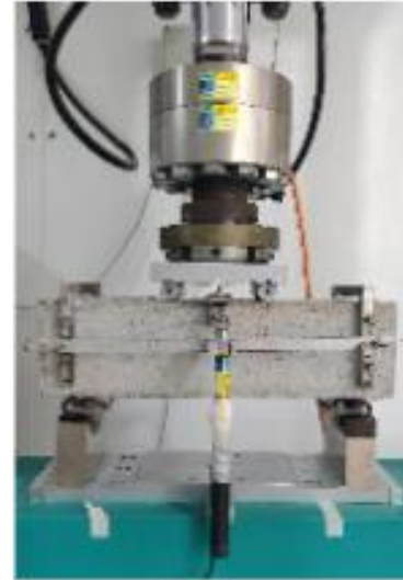
ASTM C1609/C1609M Standard test method for Flexural performance of fiber-reinforced concrete (using beam with third-point loading)
